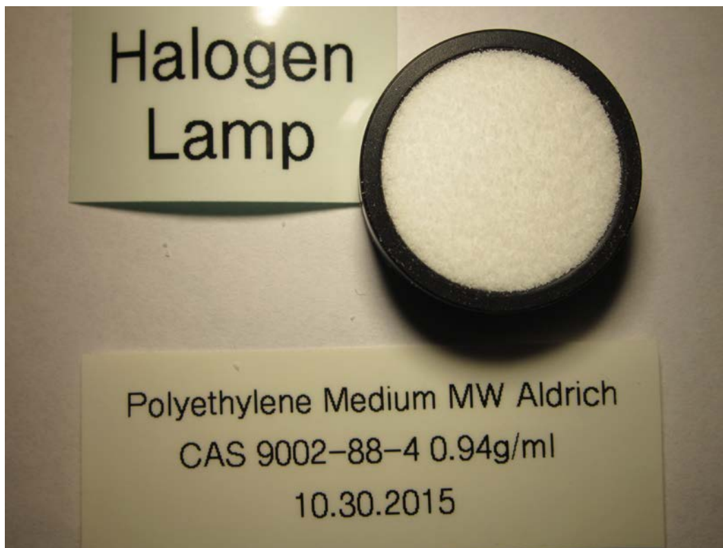
Figure 3: Polyethylene, medium density, loaded in IR sample cup.
