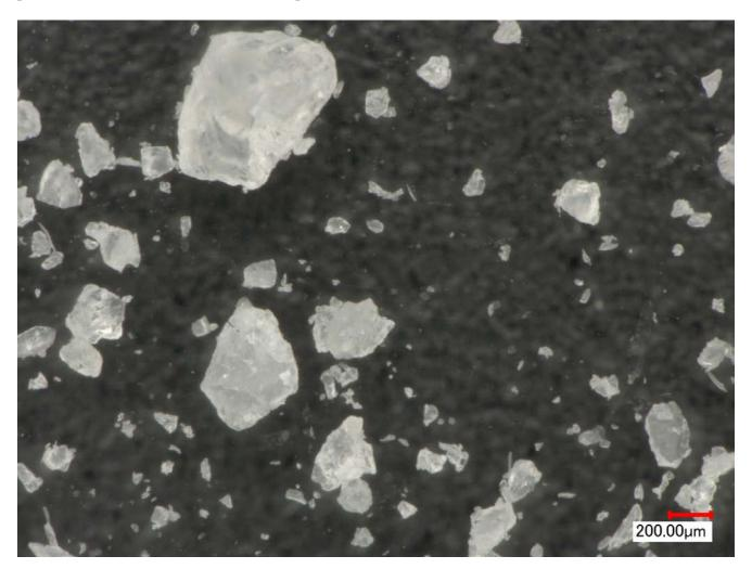
Figure 4: Photomicrograph of Polyethylene, low Mw.
