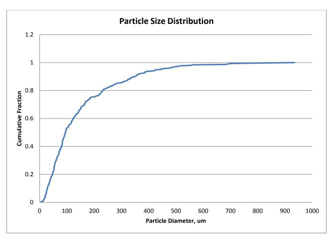
Figure 5: Particle size distribution of Polyethylene, low Mw.
