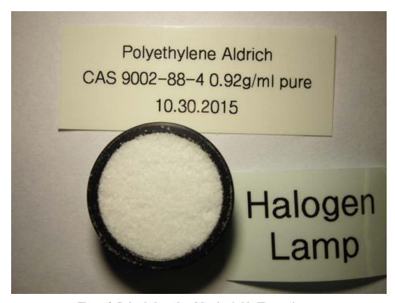
Figure 3: Polyethylene, low Mw, loaded in IR sample cup.
