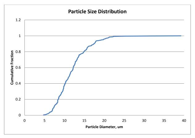
Figure 5: Particle size distribution of Poly(vinylidene fluoride).
