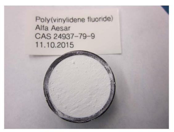
Figure 3: Poly(vinylidene fluoride) in IR sample cup.
