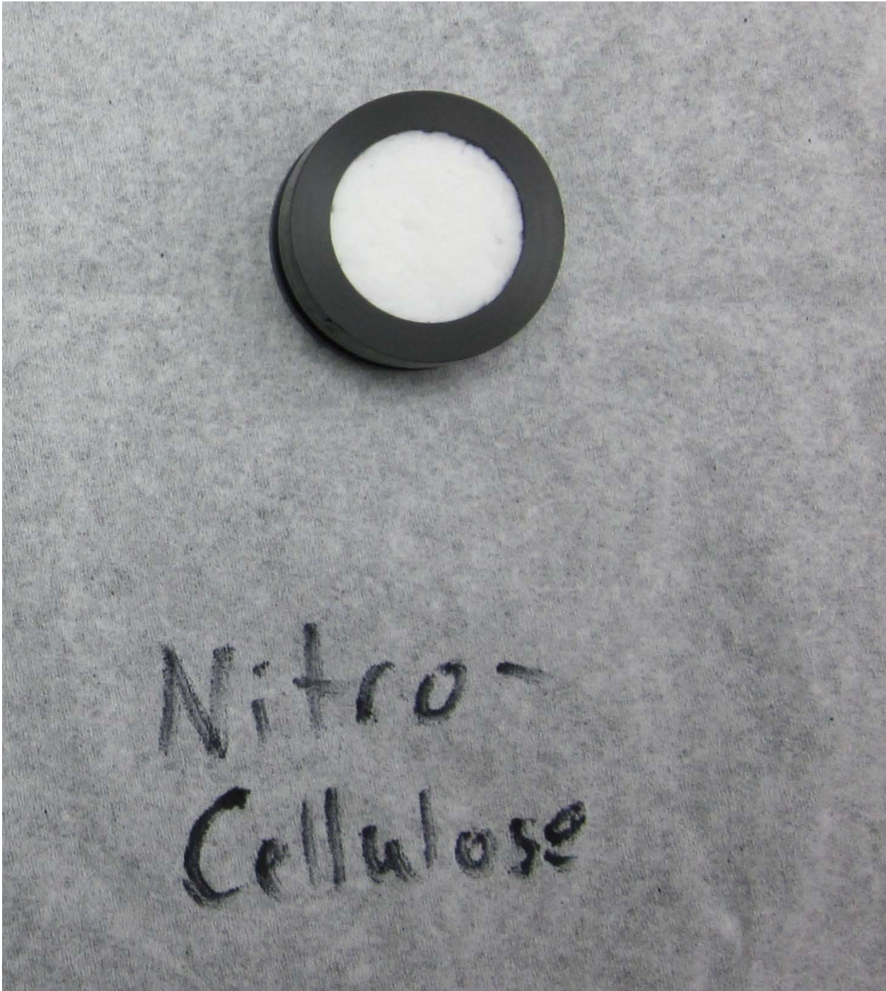
Figure2: Nitrocellulose in IR sample cup with a volume of 1.25 cm 3 .
