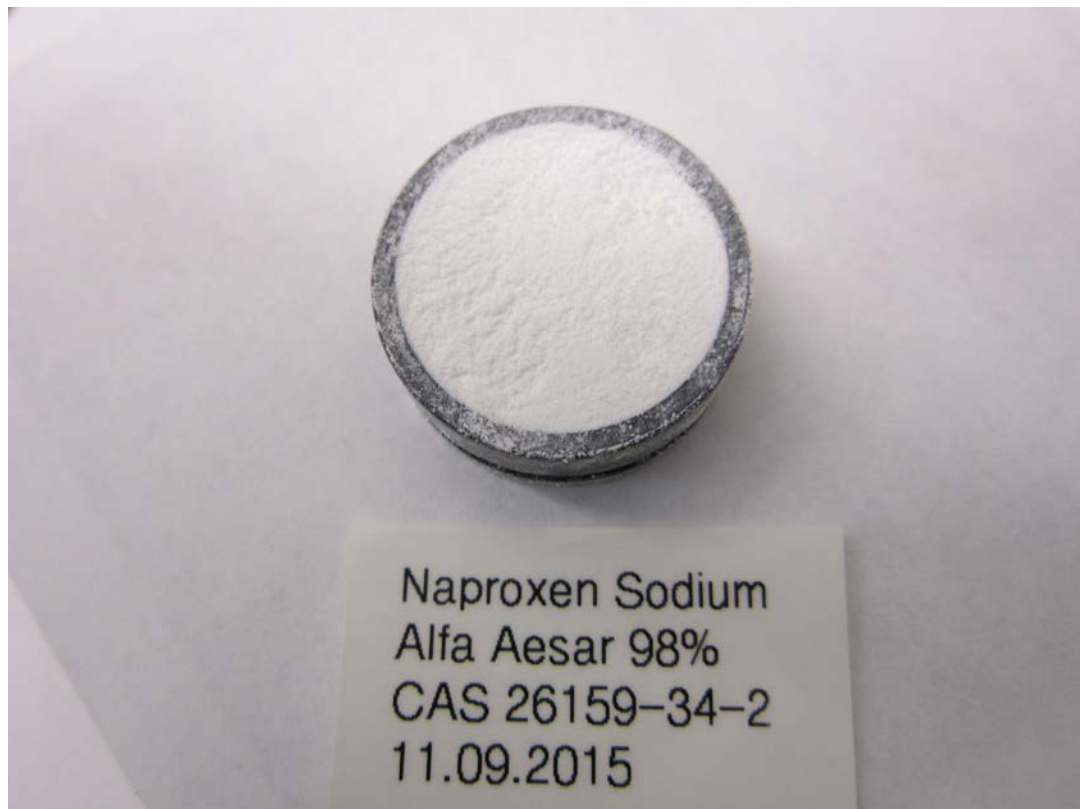
Figure 3: Naproxen sodium in IR sample cup.
