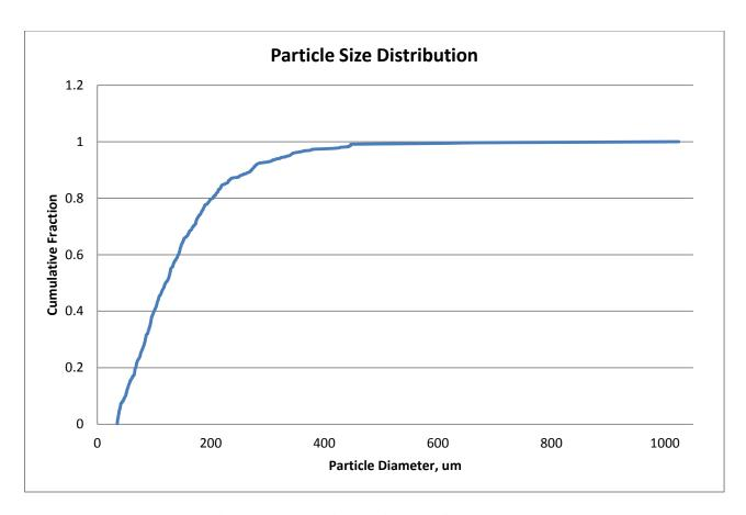
Figure 5: Particle size distribution of Monolinuron.
