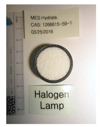
Figure 3: MES Hydrate loaded in IR sample cup.
