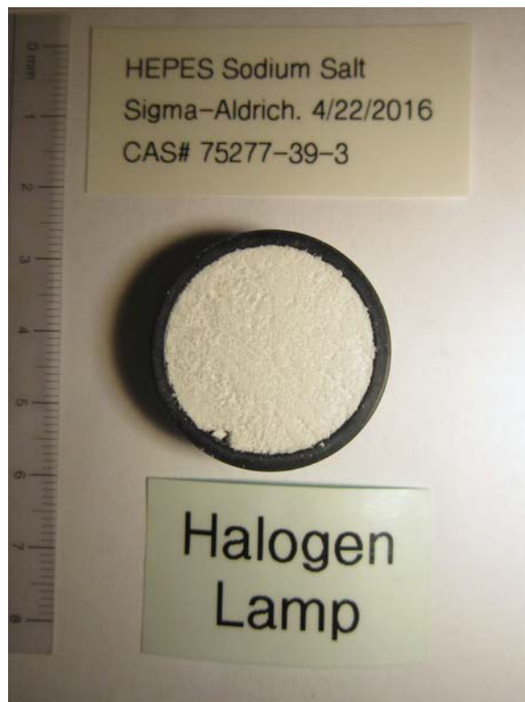
Figure 3: HEPES Sodium Salt loaded in IR sample cup.
