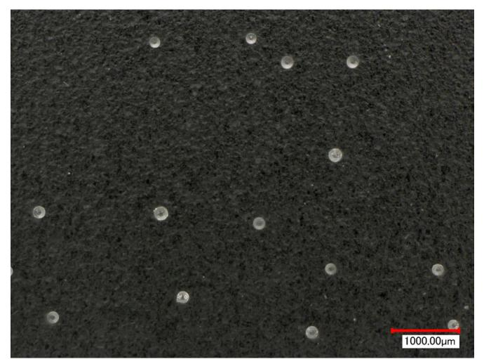
Figure 4: Photomicrograph of Glass Beads.
