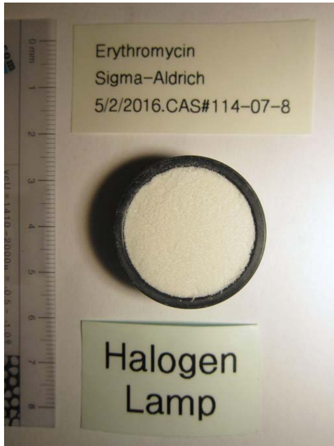
Figure 3: Erythromycin loaded in IR sample cup.
