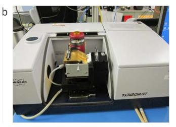
Figure 1: The Bruker 562-G integrating sphere (a) and Tensor 37 (b)
