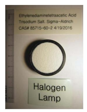
Figure 3: Ethylenediaminetetraacetic Acid Trisodium Salt loaded in IR sample cup.
