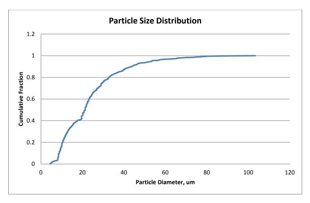
Figure 5: Particle size distribution of Ethylenediaminetetraacetic Acid Trisodium Salt.
