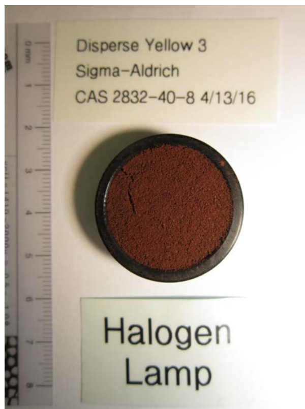
Figure 3: Disperse Yellow 3 loaded in IR sample cup.
