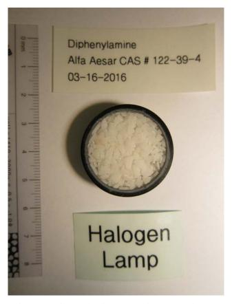
Figure 3: Diphenylamine loaded in IR sample cup.
