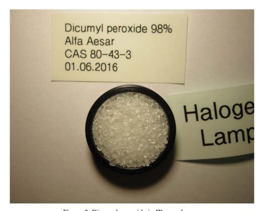
Figure 3: Dicumyl peroxide in IR sample cup.
