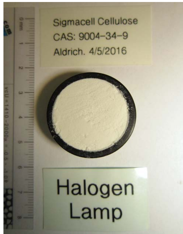
Figure 3: Sigmacell Cellulose loaded in IR sample cup.
