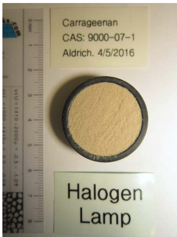
Figure 3: Carrageenan loaded in IR sample cup.
