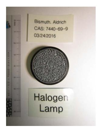
Figure 3: Bismuth loaded in IR sample cup.
