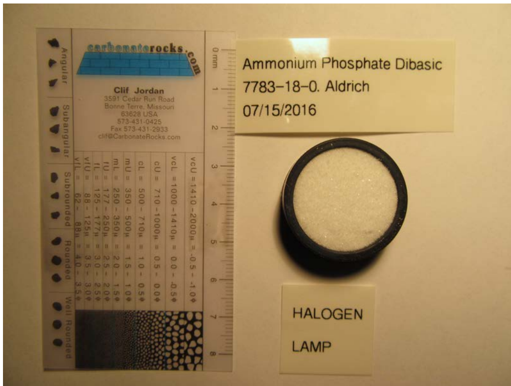
Figure 3: Ammonium Phosphate Dibasic loaded in IR sample cup.
