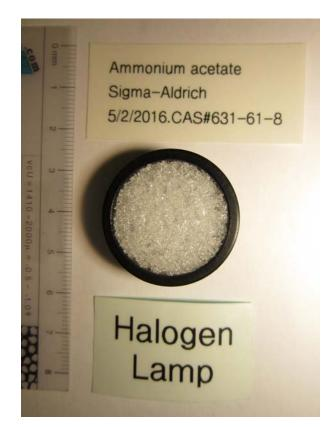
Figure 3: Ammonium Acetate loaded in IR sample cup.
