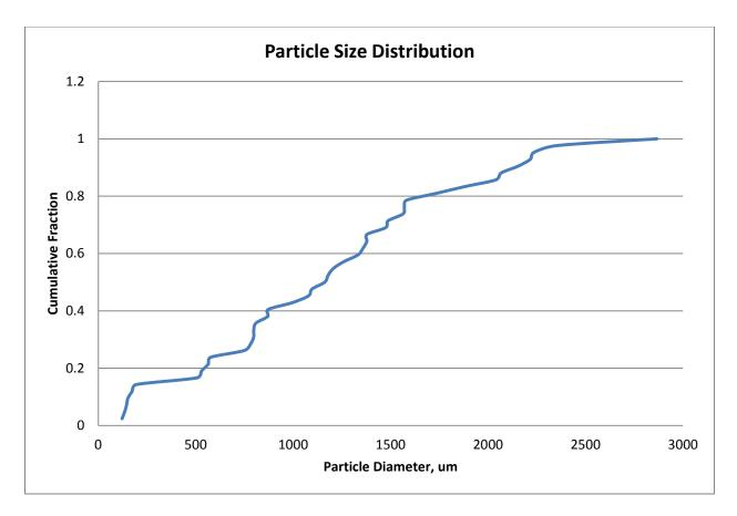
Figure 5: Particle size distribution of Ammonium Acetate.
