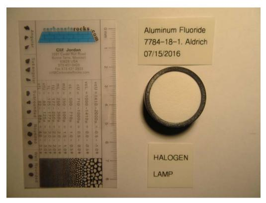
Figure 3: Aluminum fluoride loaded in IR sample cup.
