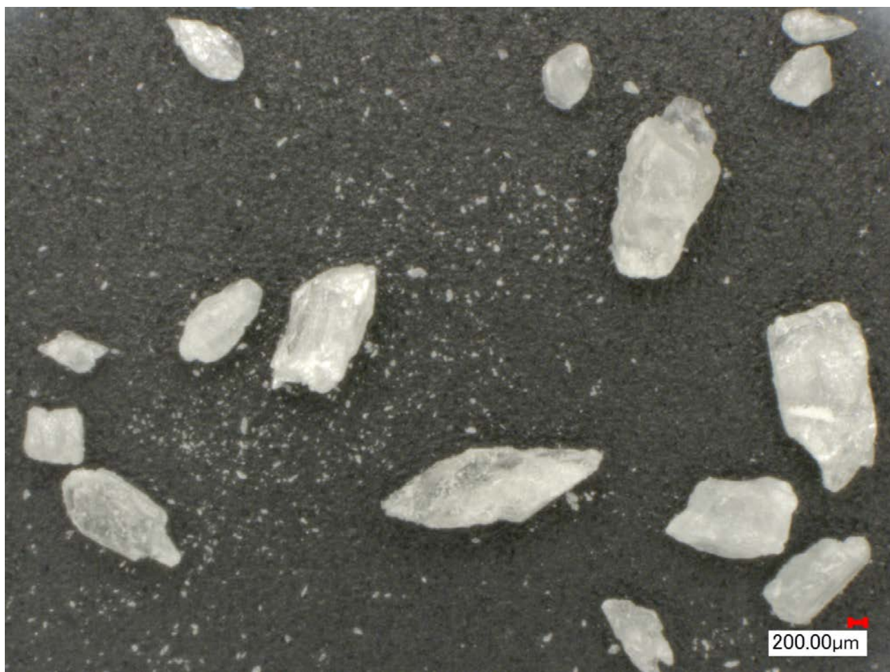
Figure 4: Photomicrograph of 2-Benzylaminopyridine crystals \geq 500 \mu\text{m} .
