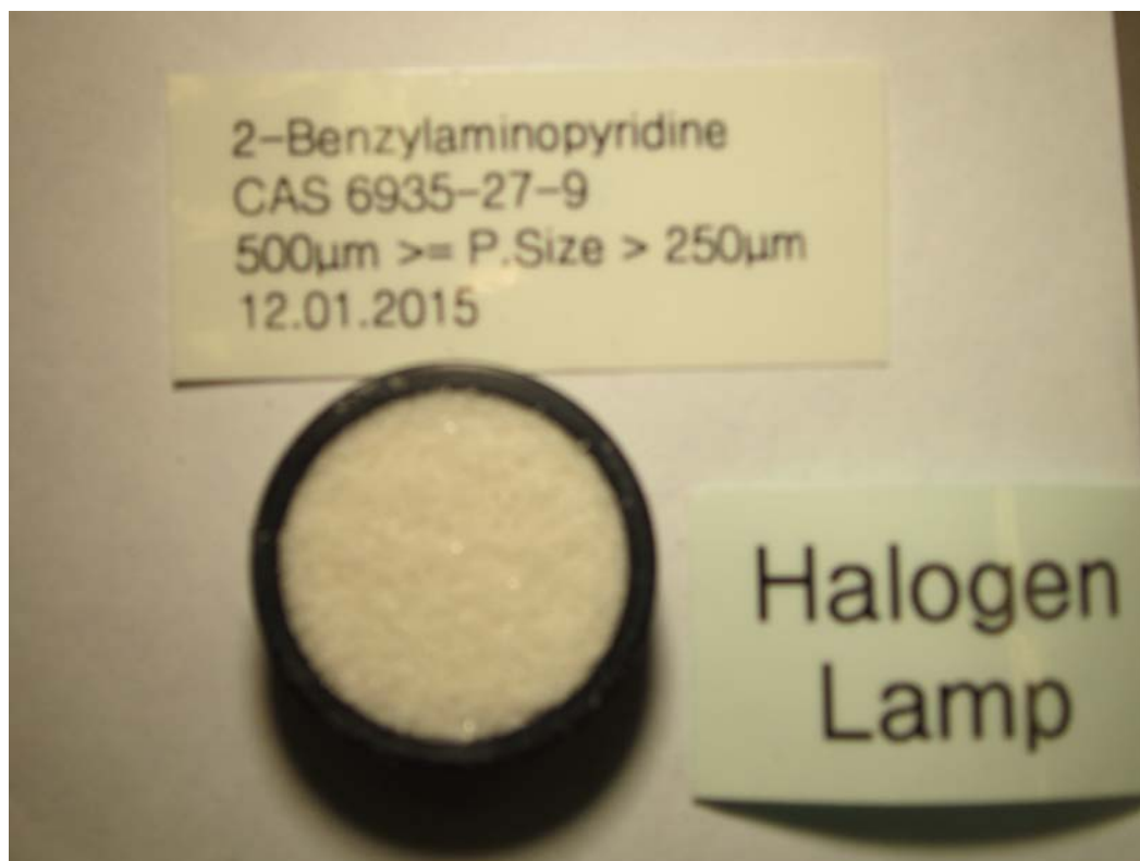
Figure 3: 2-Benzylaminopyridine 250-500 \mu\text{m} sample loaded in IR sample cup.
