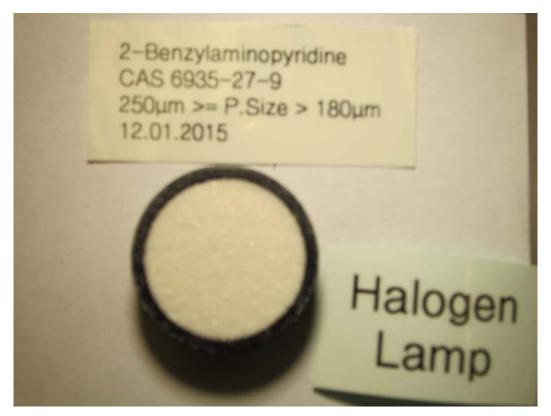
Figure 3: 2-Benzylaminopyridine 180-250 µm sample loaded in IR sample cup.
