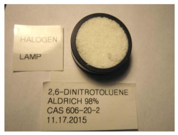
Figure 3: 2,6-Dinitrotoluene sample loaded in IR sample cup.
