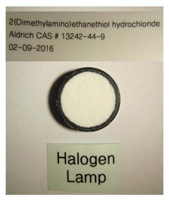
Figure 3: 2-(Dimethylamino)ethanethiol hydrochloride sample loaded in IR sample cup.
