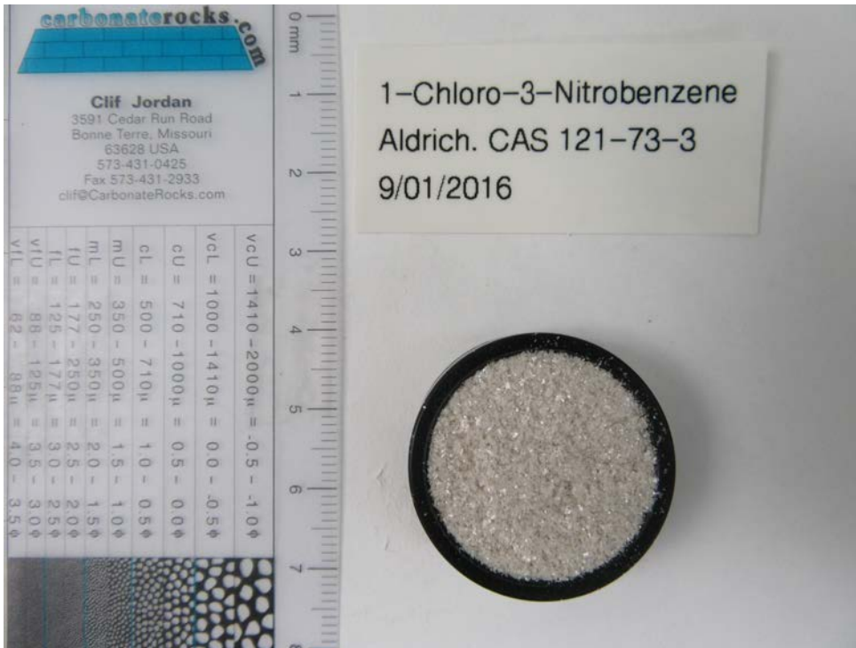
Figure 3: 1-Chloro-3-Nitrobenzene loaded in IR sample cup.
