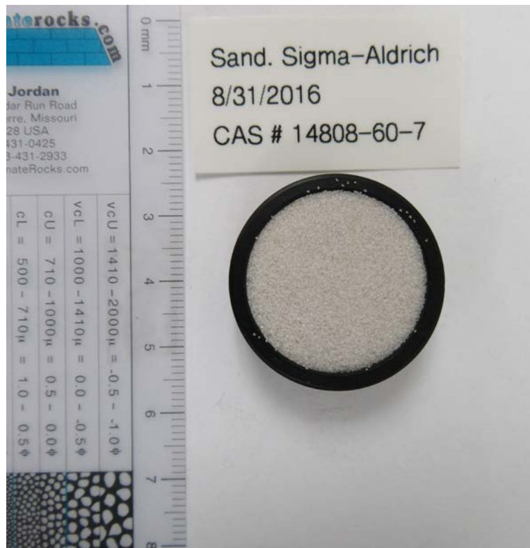
Figure 3: Sand loaded in IR sample cup.
