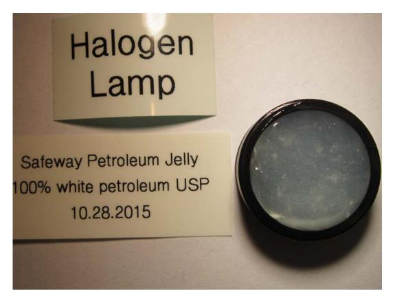
Figure 4: Petroleum Jelly loaded in IR sample cup.
