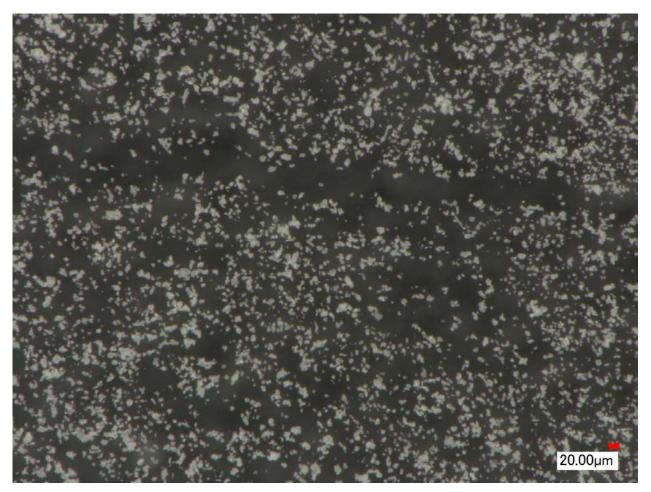
Figure 4: Photomicrograph of Soy Flour Bulk.
