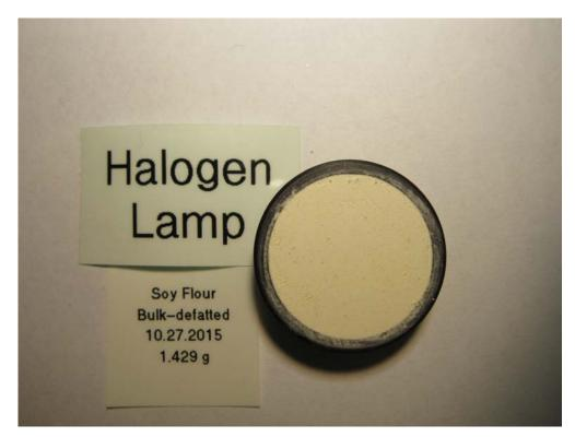
Figure 3: Soy Flour Bulk loaded into IR sample cup.
