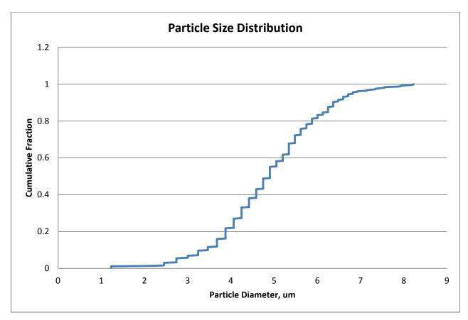
Figure 5: Particle size distribution of Soy Flour Bulk.
