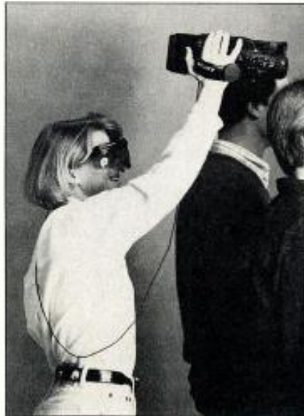
With Virtual Vision Sport, a camera operator can see the viewfinder, even if the camera is held up to shoot over a crowd.
