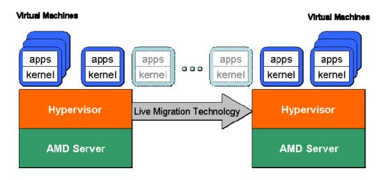
Figure 1. Live Virtual Machine Migration on AMD Processors
