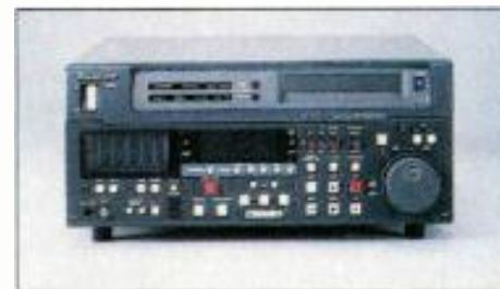
New York 1 is using its DVCPPro VTRs to dub edits onto Betacam SP tape for play-to-air.
