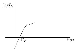
Below threshold, we observe that the current depends exponentially on the gate-source voltage, instead of quadratically (or subquadratically).
