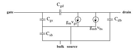
Formally, the back-gate transconductance is simply the derivative of drain current with respect to bulk-to-source voltage. In saturation, this transconductance is
