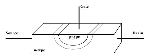
A junction FET is normally conducting, and requires the application of a sufficiently large reverse bias on the gate to shut it off. Because control is effected by altering the extent of the depletion region, such FETs are called depletion-mode devices.
