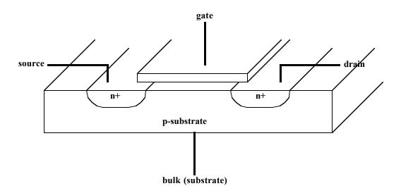
As an increasing positive voltage is applied to the gate, holes are progressively repelled away from the surface of the substrate. At some particular value of gate voltage (the threshold voltage  $V_t$ ), the surface becomes completely depleted of charge. Further increases in gate voltage induce an *inversion layer*, composed of electrons supplied by the source (or drain), that constitutes a conductive path ("channel") between source and drain.
