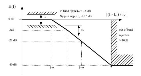
Figure 2-13 QPSK Upstream Transmitter Power Spectrum
