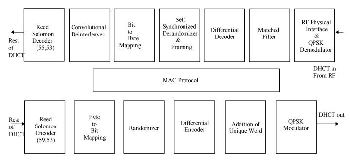
Figure 2-3 DHCT OOB Transceiver Conceptual Block Diagram
