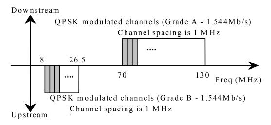
Figure 2-1 Spectrum Allocation For the Bi-directional PHY on Coax
