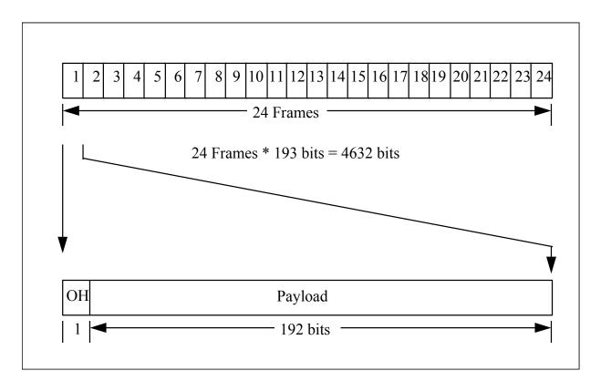
Figure 2-5 SL-ESF Frame Structure
