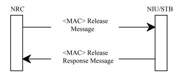
Figure 2-20 Connection Release Signaling
