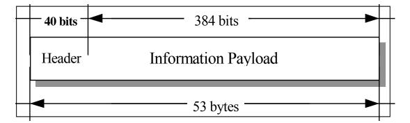
Figure 2-12 ATM Cell Structure
