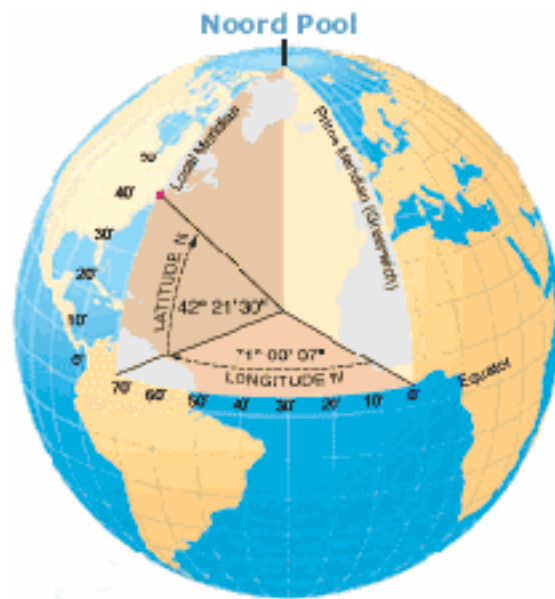
Figure 1-3 How the latitude and longitude at any one point on Earth is measured.
