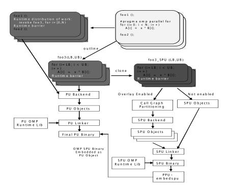
Figure 1 Code generation process
