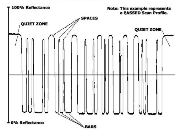
Figure 2 - Passing Scan Reflectance Profile
