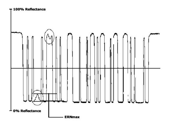
Figure 14 - Grade 4/A Defects
