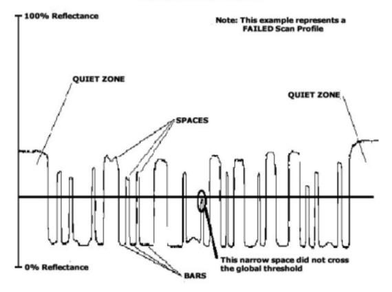
Figure 3 - Failed Scan Reflectance Profile
