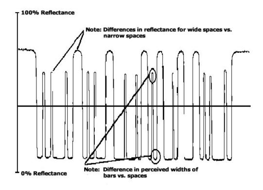
Figure 12 - Grade 4/A Modulation
