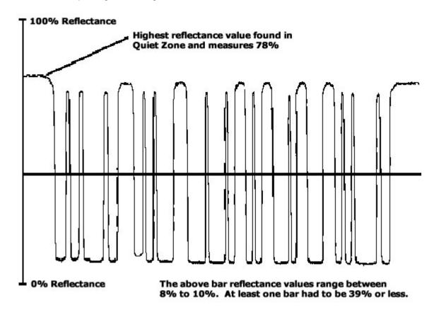
Figure 6 - Passing Minimum Reflectance Test
