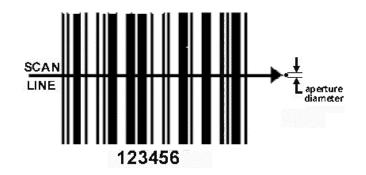
Figure 1 - Scan Line through a Bar Code
