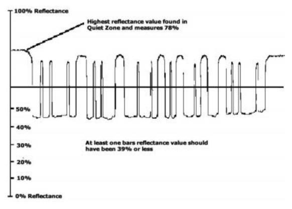
Figure 7 - Failing Minimum Reflectance Test
