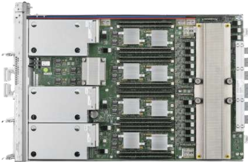
Figure 15. Each CMIU board contains a SPARC M7 processor, 16 DDR4 DIMM slots, an I/O controller ASIC, and three PCIe x16 hot-pluggable carriers.
