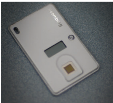
BLAW's dedicated biometric fingerprint scan device—known as a Bloomberg B-Unit—allows users to log in via any Internet-connected computer anywhere in the world.
