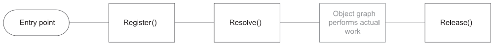
Figure 3.12 In a single-threaded application, each method will tend to be invoked only once. Configuration of the container is immediately followed by composing the application’s object graph that performs the actual work. When the work is completed, the Release method is invoked before the application exits.
