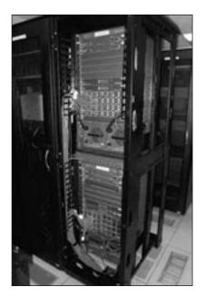
Figure 4. A pair of Catalyst 6500 Core Routers located in our networking lab during testing, with their single mode fiber optic cable connections active.
