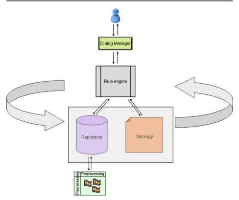
Fig. 1 Abstract model of the architecture of the MashUp Tool
