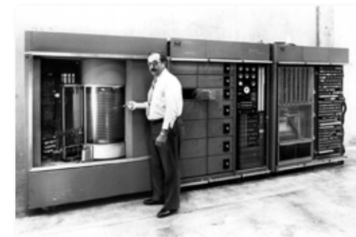
1956 IBM 350 RAMAC DISK STORAGE UNIT The original hard disk drive, the IBM 350 RAMAC Disk Storage Unit, stores five megabytes of data on 50 magnetic disks, each 24 inches in diameter. The disks spin at 1200 rpm, and read-write heads locate and access data on the disks in less than one second. RAMAC stands for "Random Access Method of Accounting and Control," a name that wins out over rejected labels for the system — DREAM (Direct Reference Electronic Accounting Machine) and UNCLE (Universal Numeric Calculating and Logic Engine).
