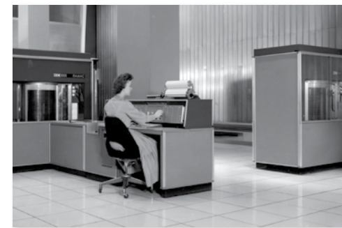
1956 IBM 305 RAMAC SYSTEM The IBM 350 RAMAC Disk Storage Unit is a major component of the larger IBM 305 RAMAC system — a flexible, electronic, general-purpose data processing machine that enables businesses to record transactions as they occur. The system maintains records on a realtime basis, provides random access to any record, eliminates peak loads and simultaneously produces output by either print or punch cards.
