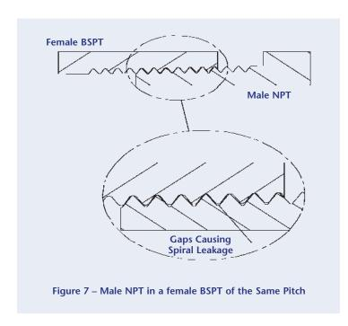
Chemical attack can occur when improper thread sealants are used. Thread sealing is an attempt to block the spiral leak path which occurs when the crests and roots of the thread forms do not match. Anaerobic thread sealants should be avoided when sealing plastic thread forms. These sealants contain chemicals which may attack plastics. Use of a Teflon-based pipe thread sealant is a better choice for plastic threads.
