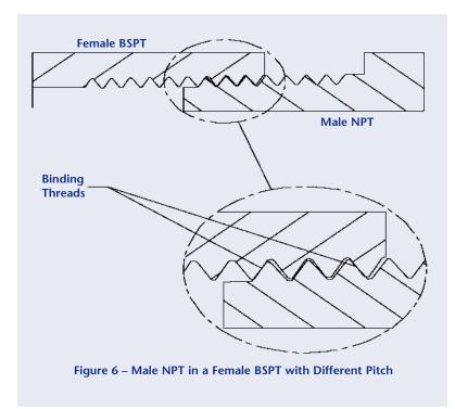
Another tapered thread is the British Standard Pipe taper, or BSP, covered by British Standard 21. BSP thread is commonly used for low pressure plumbing, but is not recommended for medium and high pressure hydraulic systems. This form uses the Whitworth thread with an angle of 55° and a 1 in 16 taper. It is not interchangeable with the American NPT thread, though at the 1/2" and 3/4" size, they both have 14 threads per inch.
