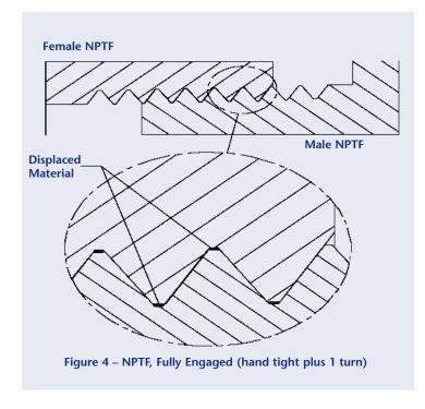
thread. See figure 2. This offers more threads a chance of sealing against spiral leakage. Crest and root control is still missing, but with thread sealant, a pressure tight joint would be easier to accomplish.
