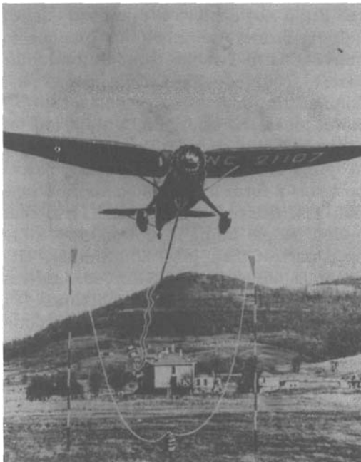
Figure 5.2 Air mail pick up and delivery in 1944. The mail container rests on the ground between two poles.
