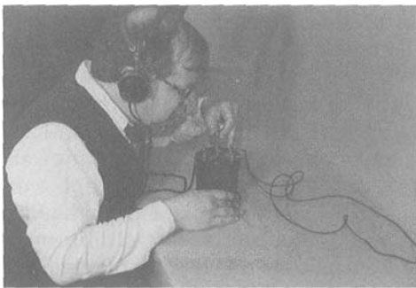
Figure 3.17 A crystal-and-catwhisker radio, 1922. A tiny wire was touched to the "sweet spot" on a galena crystal to bring in a station. (Courtesy Pavek Museum.)
