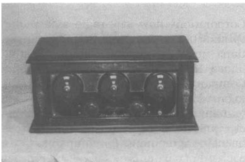
Figure 4.7 A Holmes-Jordan radio with three tuning stages, 1925. Three types of batteries were needed, including a lead acid car-type battery. Acid burns in carpets were common. (Courtesy Pavek Museum.)
