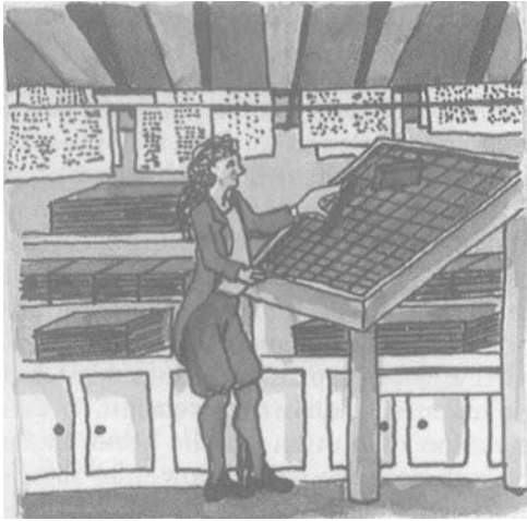
Figure 2.4 Type was chosen from a job case and set by hand.
