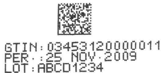
Figure 3.2.2-1 Inkjet printed GS1 DataMatrix
