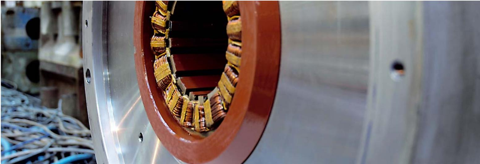
A substantial share of Siemens' current production of compressor trains is fitted with so-called active magnetic bearings (AMB). A glimpse into their concept and performance reveals the appeal of computer-controlled magnetic attraction.
