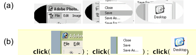
Figure 10: Converting a Graphstract [7] (a) to a Sikuli script (b).
