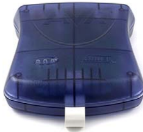
Figure 4. JTAGICE mkII also functions as an on-chip debugger.
