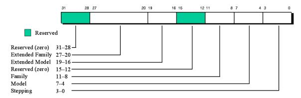
Figure 1. Format of CPUID Value Returned by Function 1
